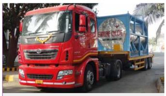
Improving Ethylene Oxide (EO) Transportation Safety At our Thane manufacturing site in India, we have identified EO transportation as a key process safety risk because of the 300km distance that EO has to be transported to the site, the conditions on India's busy roads and the local standards of tanker equipment. We have adopted a comprehensive safety approach that includes:
